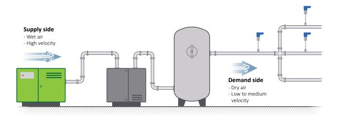
Measure dry and clean gas only for correct measurements and a long lifetime.
